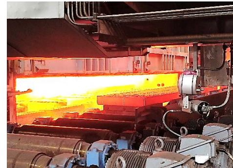
Slab Extraction in HSM at JVML-Vijayanagar
