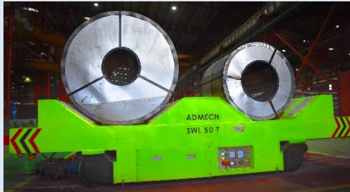
Li-ion battery operated coil transfer cars at JSW Steel Coated plants to reduce emissions
