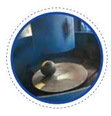
**Impact Test:**Ball Drop Test.
