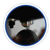
**Hardness Test:**Average Surface HRc, Average Volumetric HRc.
