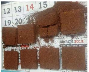
Fig VII: Direct Shear test
