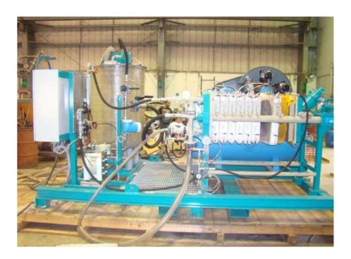
Fig. 2.9 Pilot scale pressure filter set up
