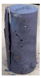
Figure V. Determining UCS of rock sample
