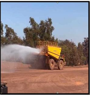
Water Tanker Arrangement (16KL & 50KL water sprinkler) for Haul Road Dust Suppression
