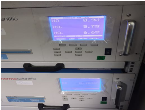
Installation of NO 2 & CO analyzers at CAAQMS 2, 3, 4
